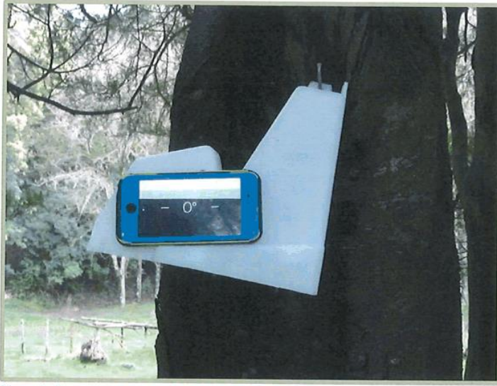
Photo 1: Base plate level on a side set (Photo J Hart)
